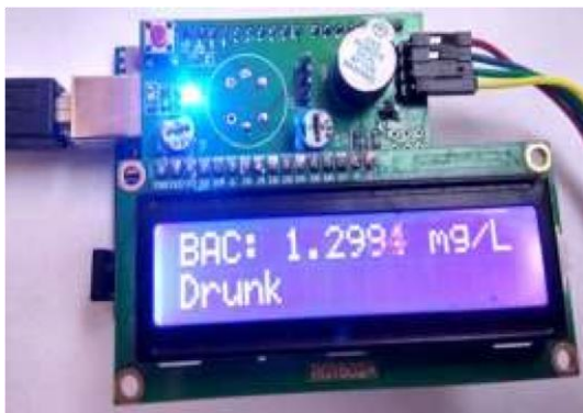
Figure 7 LCD Output of alcohol detection when driver is drunken state
