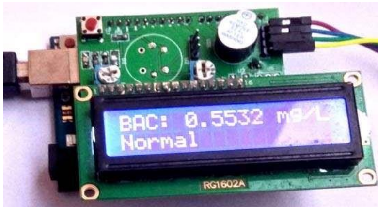
Figure 6. LCD Output of alcohol detection when driver is not in drunken state
