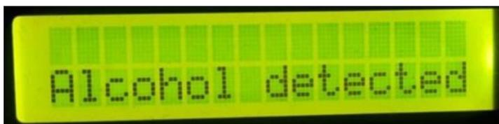
Fig 4.2.2 When Alcohol is detected
