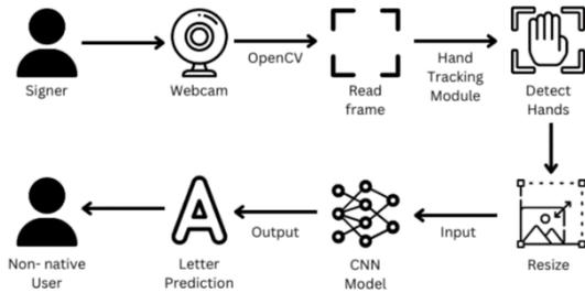
Fig. - 2 System Architecture Diagram
