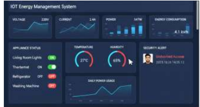
Fig 4. Web-based real-time smart home monitoring dashboard
