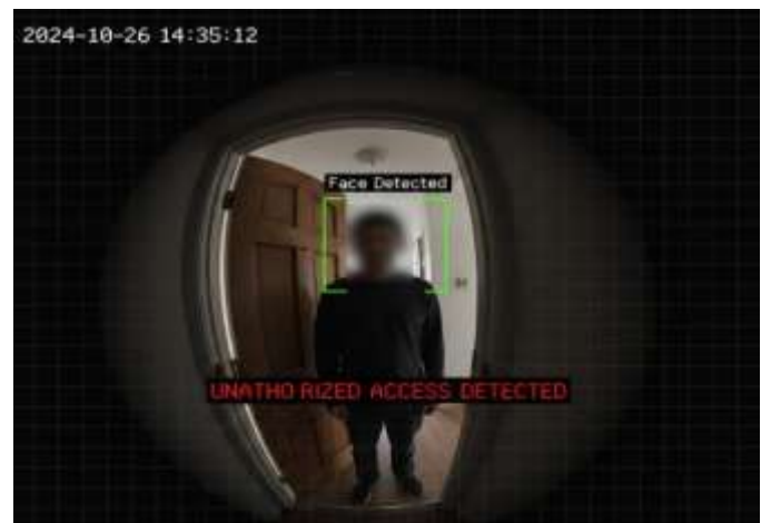
Fig 5. Unauthorized face detection and alert generation
