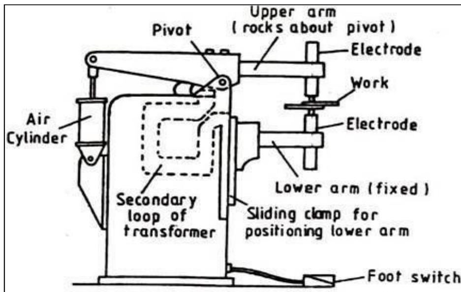
The concept of heat generation can be stated by using a modification of Ohm's law i.e. when current passes through a conductor then the electrical resistance of the conductor will oppose the current flow and results in heat generation as
