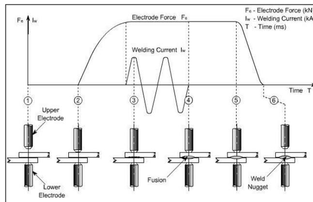
**The contact area of electrodes:** contact area of the face of electrodes affects the weld size and shape which can be varied by varying the electrode tip.
