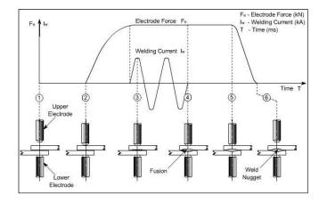
The contact area of electrodes: contact area of the face of electrodes affects the weld size and shape which can be varied by varying the electrode tip.
