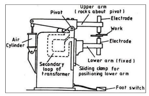
The concept of heat generation can be stated by using a modification of Ohm's law i.e. when current passes through a conductor then the electrical resistance of the conductor will oppose the current flow and results in heat generation as  $\mathbf{H} = \mathbf{I}^2 \mathbf{D}$
