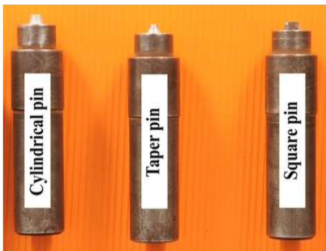
Figure 2 FSW Tools equipped with its pins
