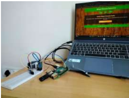
Figure 3 : Hardware Setup of Wheat Disease Detection System
