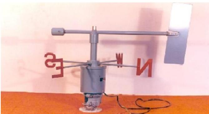
Fig. 3: Potentiometric wind vane
