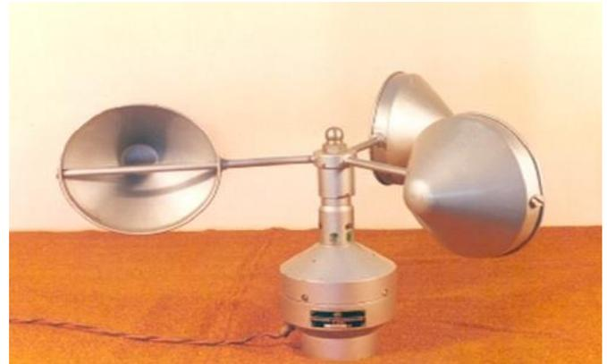
Fig. 4: Three-Cup chopper anemometer
