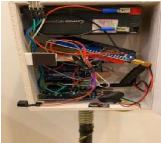
Fig 6.2 Smart stick and GPS Tracking system in the box
