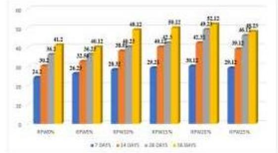
**Compressive strength of concrete with mix design of M30 @ 4% Nano Silica**
