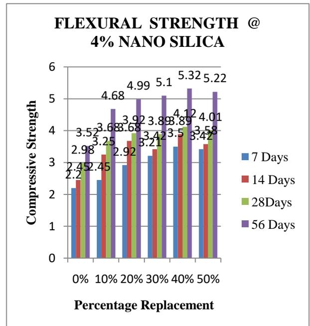
**Fig.: 6.2. FLEXURAL STRENGTH @ M20 4% NANO SILICA**
