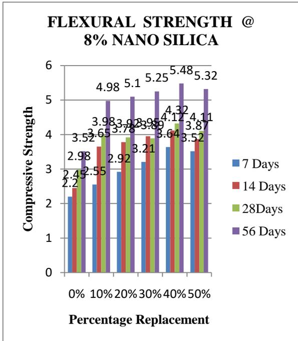
Fig.: 6.3. FLEXURAL STRENGTH @ M20 8% NANO SILICA
