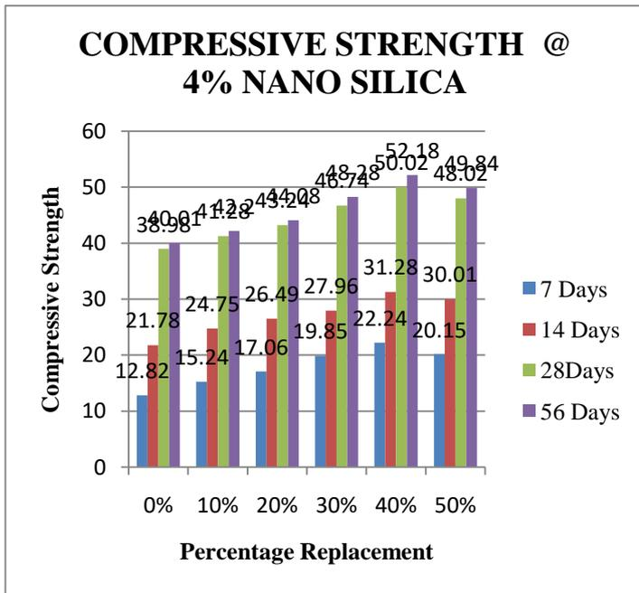
Fig.: 6.5. COMPRESSIVE STRENGTH @ M30 4% NANO SILICA
