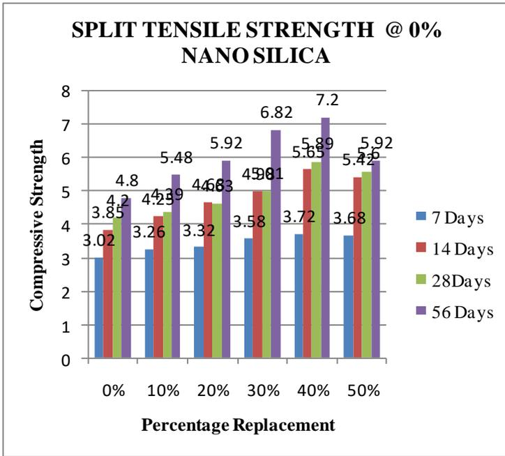
Fig.: 6.1. SPLIT TENSILE STRENGTH @M20 0% NANO SILICA
