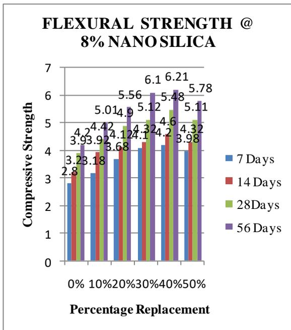
Fig.: 6.6. FLEXURAL STRENGTH @ M30 8% NANO SILICA
