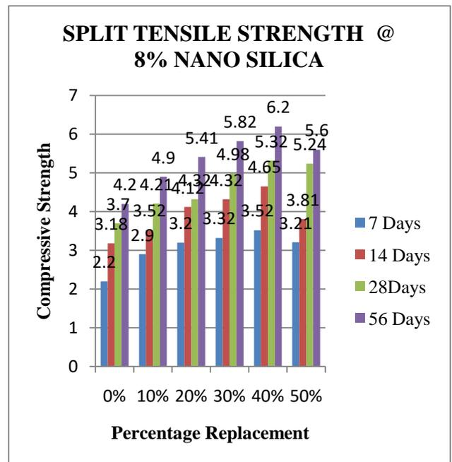
Fig.: 6.6. SPLIT TENSILE STRENGTH @ M30 8% NANO SILICA
