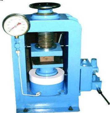
Fig. 1 Compressive Strength Test
