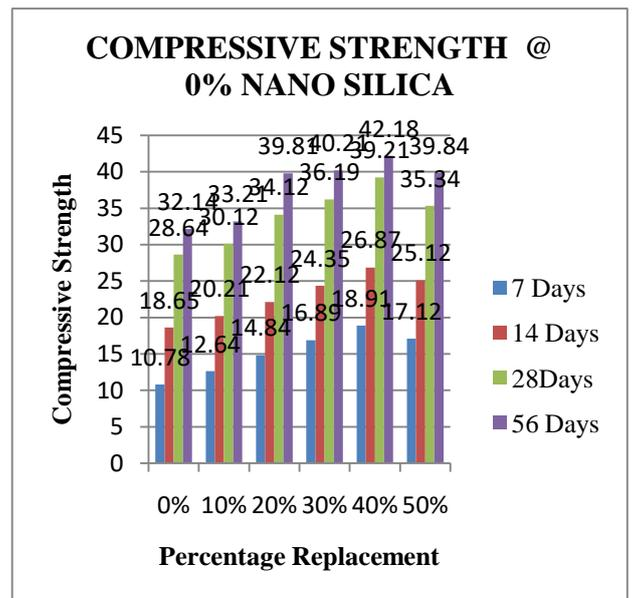
**Fig.: 6.1. COMPRESSIVE STRENGTH @ M20 0% NANO SILICA**
