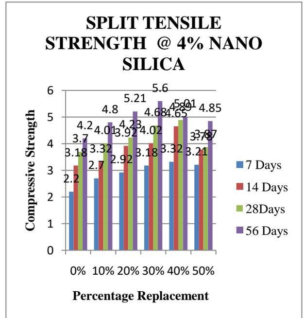
Fig.: 6.5. SPLIT TENSILE STRENGTH @ M30 4% NANO SILICA
