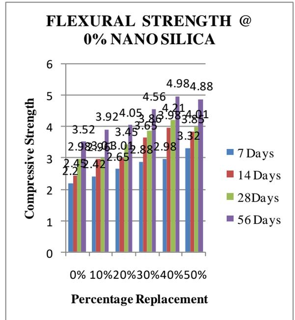
**Fig.: 6.1. FLEXURAL STRENGTH @ M20 0% NANO SILICA**
