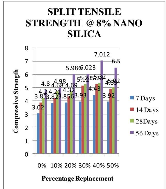
Fig.: 6.3. SPLIT TENSILE STRENGTH @ M20 8% NANO SILICA
