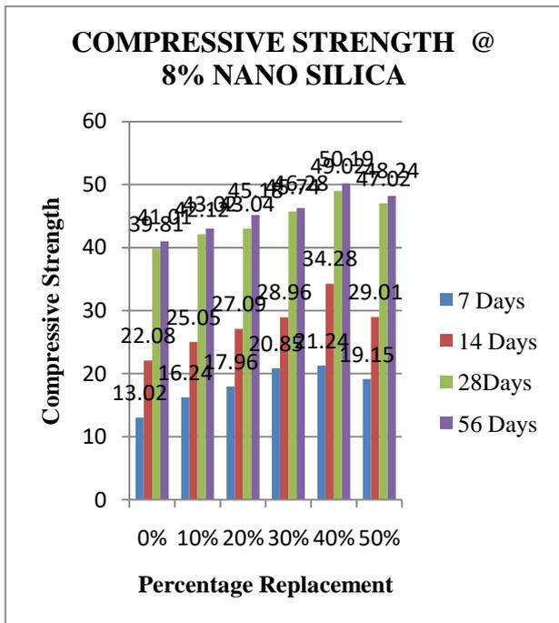
Fig.: 6.6. COMPRESSIVE STRENGTH @ M30 8% NANO SILICA
