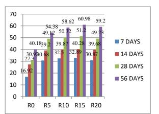
5.4 COMPRESSIVE STRENGTH OF CONCRETE WITH MIX DESIGN OF M40@ RHA(0%,5%,10%,15%,&20%)+GLASS FIBER(1.5%)
