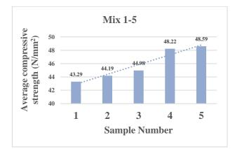
Fig. 1: Average compressive strength  $(N/mm^2)$
