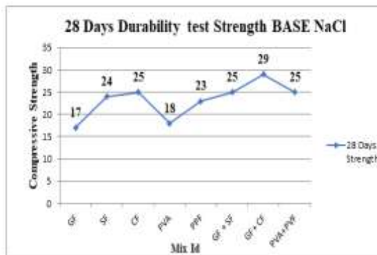
Fig.:10. Compressive Strength of fibers Durability (NaCl) @ 28 days
