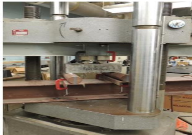
Fig 5.8 Flexural Beam Test Setup
