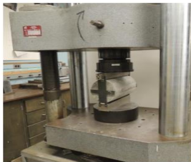
Fig 5.7 Split Tensile Strength Setup.
