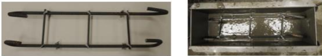
Fig 5.9 Reinforcement and Framework for RFC Beam
