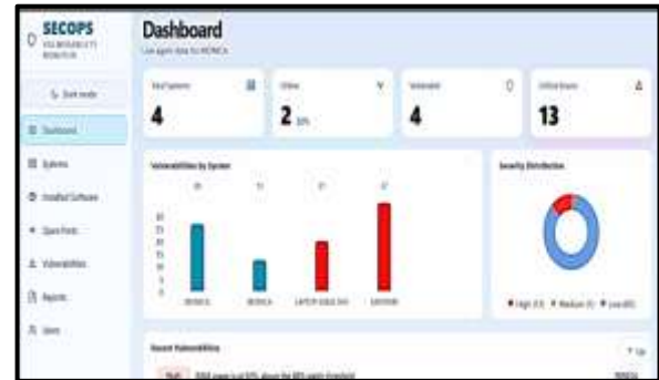
Figure 1. Centralized Dashboard showing system counts, vulnerability distribution by host, and overall severity breakdown.
