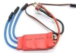
Figure 4.7.1 electronic speed controller
