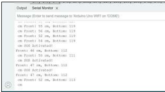
FIGURE 10: Front and bottom distance readings(in cm) and SOS activation.
