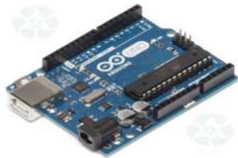
FIGURE 2: Arduino Uno (ATmega328 Microcontroller)
