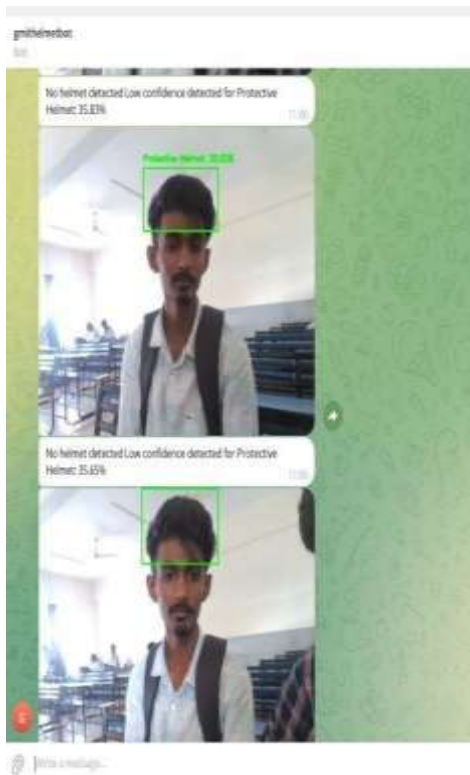
Figure 2 : Helmet rules violation being detected
