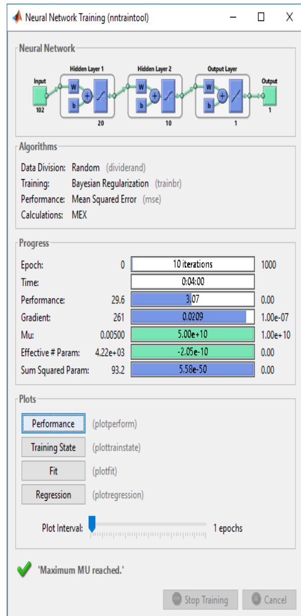
Fig.7 Designed Neural Network and its training parameters
