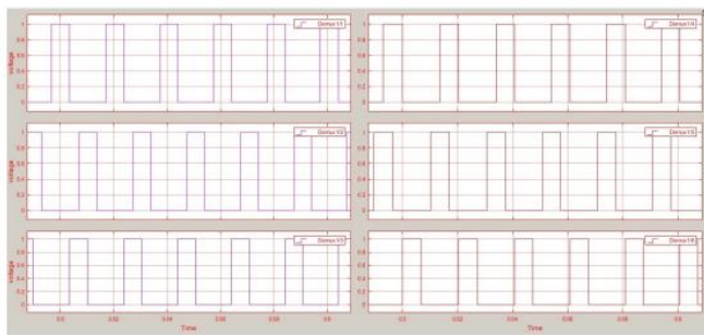
Figure 3.8: gating pulse for inverter
