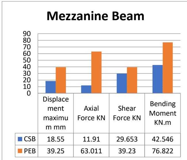
Fig no. 10 Results for mezzanine beam of CSB and PEB
