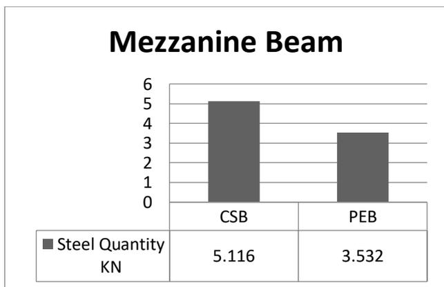
Fig no. 6.8 Steel quantity for mezzanine beam of CSB and PEB
