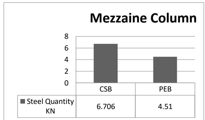
Fig no. 8 Steel quantity mezzanine column of CSB and PEB
