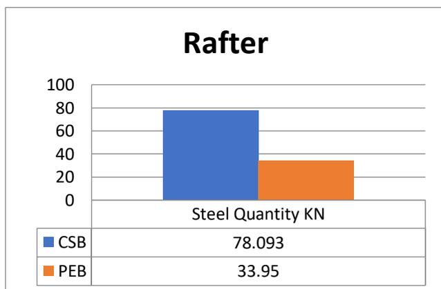
Fig no. 14 Steel quantity for rafter of CSB and PEB
