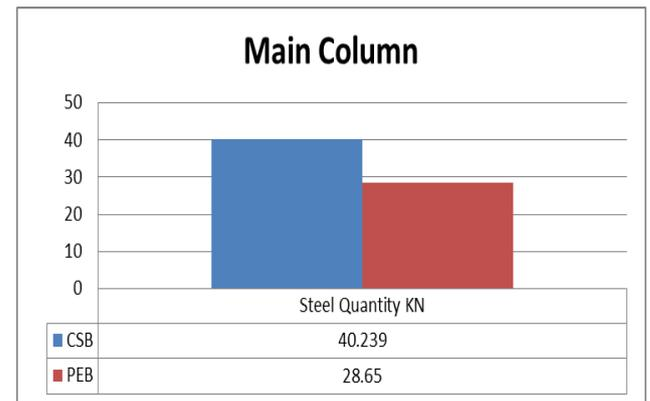
Fig no. 4 Steel quantity for main column of CSB and PEB
