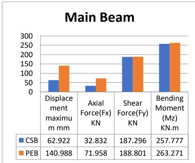
Fig no. 6 Results for main beam of CSB and PEB
