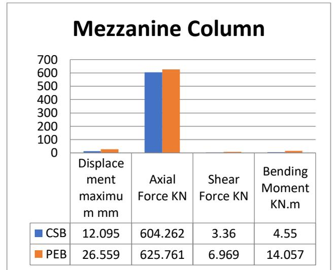
Fig no. 9 Results for mezzanine column of CSB and PEB
