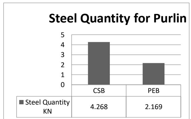
Fig no. 12 Steel quantity for purlin of CSB and PEB
