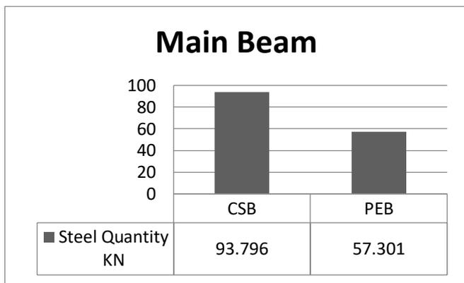
Fig no. 7 Steel quantity for main beam of CSB and PEB
