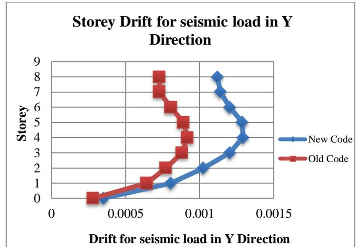
**Fig- 7:** Maximum Storey Drift for Seismic load in Y direction
