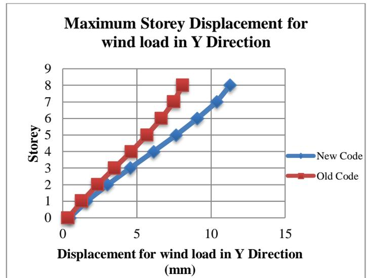
Fig- 9: Maximum Storey Displacement for Wind load in Y direction
