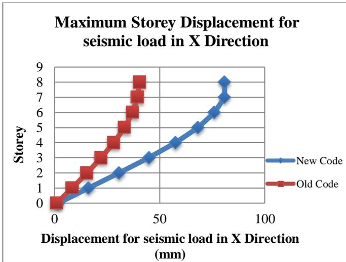
Fig- 4: Maximum Storey Displacement for Seismic load in X direction
