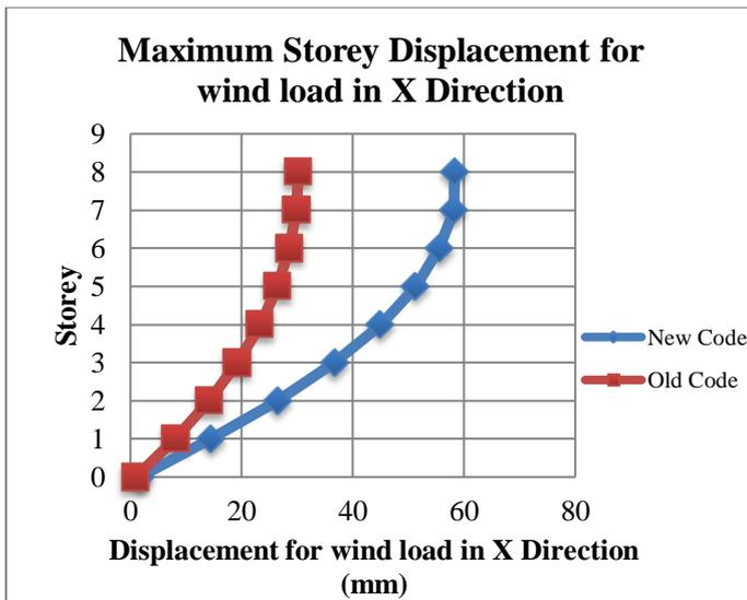
Fig- 8: Maximum Storey Displacement for Wind load in X direction
