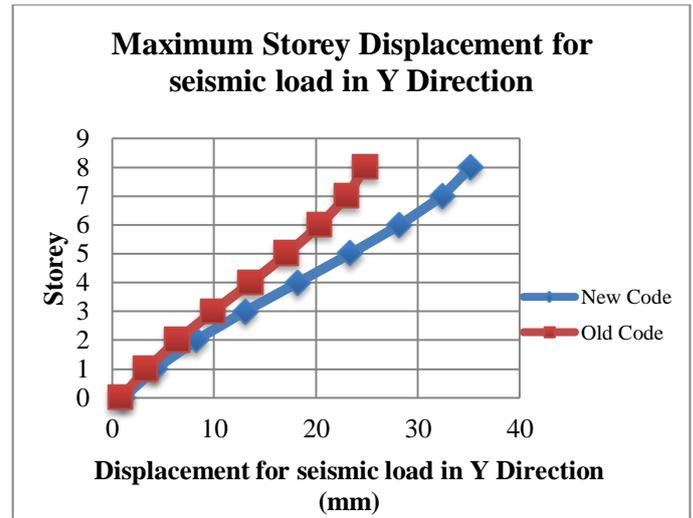
Fig- 5: Maximum Storey Displacement for Seismic load in Y direction
