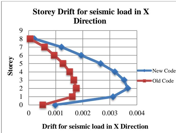
**Fig- 6:** Maximum Storey Drift for Seismic load in X direction
