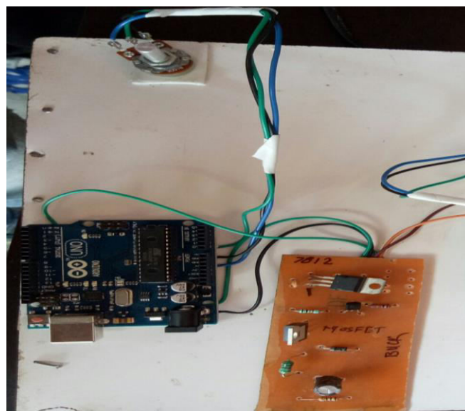
Fig5 (f). Hardware setup of buck converter with arduino.
