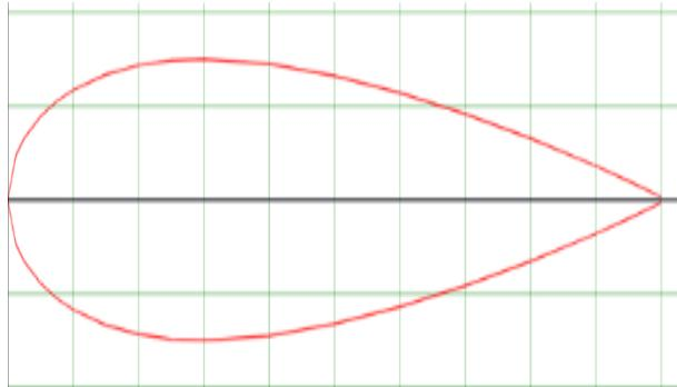
**Fig.4 NACA 0015****9. Domain's Geometry:**
