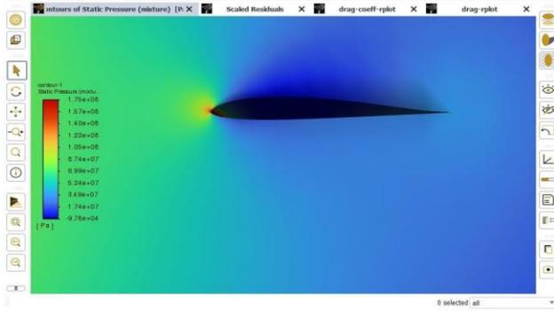
**Fig.5 Pressure contour of hydrofoil without appendage**
