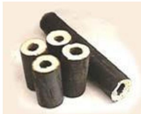
Fig.4.3 Briquette made by screw extruder
