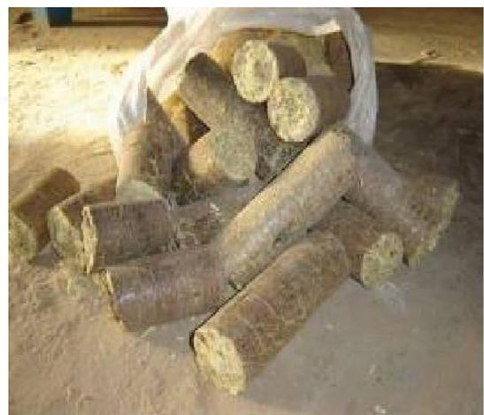
Fig. 4.6 Briquettes made by hydraulic press
