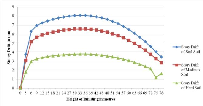
Fig. 3.1 Storey Drift along Z direction for different Soil Conditions
