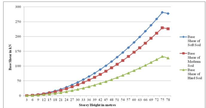
Fig. 3.3 Base Shear of Different Storey
