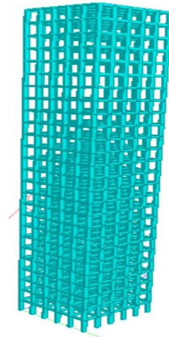
**Fig. 2.2** Isometric 3D View of G+25 Building
