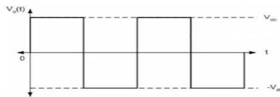
Fig-10: Square wave output of Inverter
