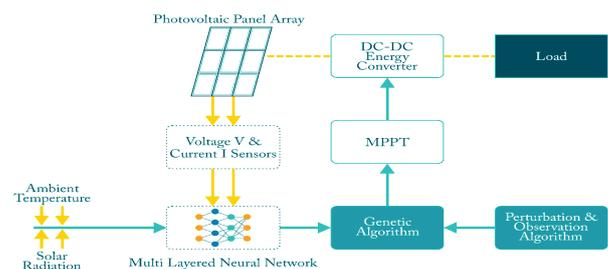
Fig-11: Block Diagram of proposed Neural Network (AI) system
