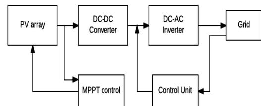
Fig-1: Block Diagram of Solar System with MPPT Based Inverter and Grid Synchronization
