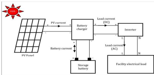
Fig-3: Configuration of the Stand-Alone PV System
