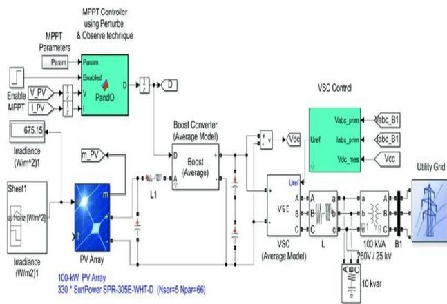
Fig-12: Modeling and Simulation of Solar System with MPPT Based Inverter and Grid Synchronization
