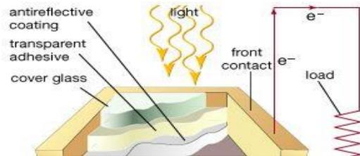
Fig-4: Summary on how solar cells work
