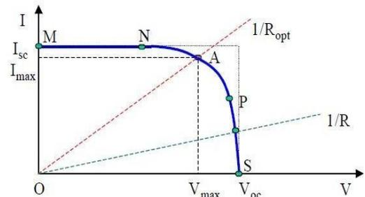
Fig-7: A typical current-voltage (I-V) curve for a solar cell.
