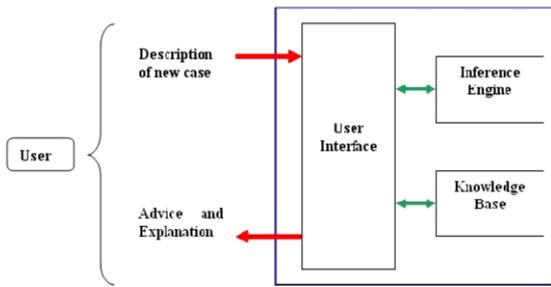
Fig-2: Block diagram of expert system
