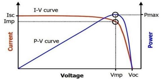
Fig-6: Characteristic I-V curve of a practical photovoltaic device
