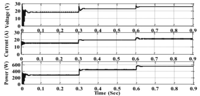
Fig-14: waveform of PV output
