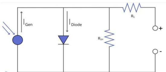
Fig-5: Equivalent Circuit for Solar Cell
