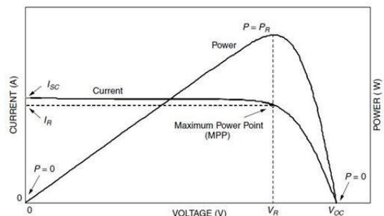
Fig-8: MPPT in I-V Curve and P-V Curve
