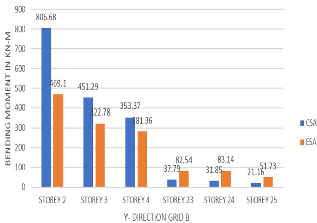
Fig -8: Bending Moment of Beams Along Storey model 2
