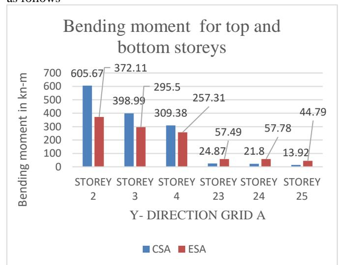
**Fig -7:** Bending Moment of Beams Along Storey model 1
