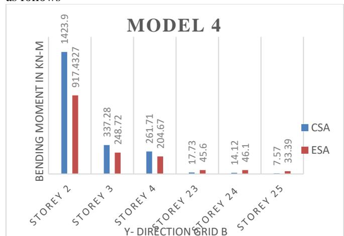
Fig -10: Bending Moment of Beams Along Storey model 4
