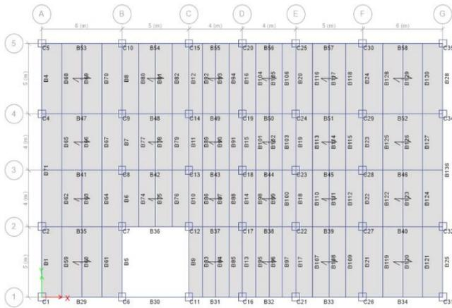
Fig -3: 2D Plan View of Steel Model 3 At Storey 2
