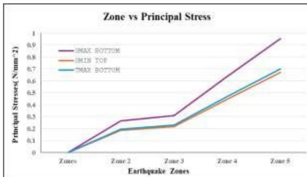
**Fig. 10.6: Principal stress across varying Earthquake Zones**
