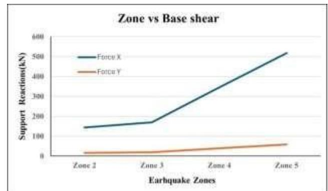
**Fig. 10.2: Base Shear across varying Earthquake Zones**
