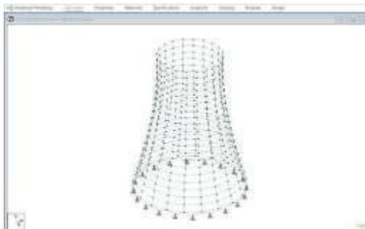
**Fig. 2: Analytical model of a Cooling tower**
