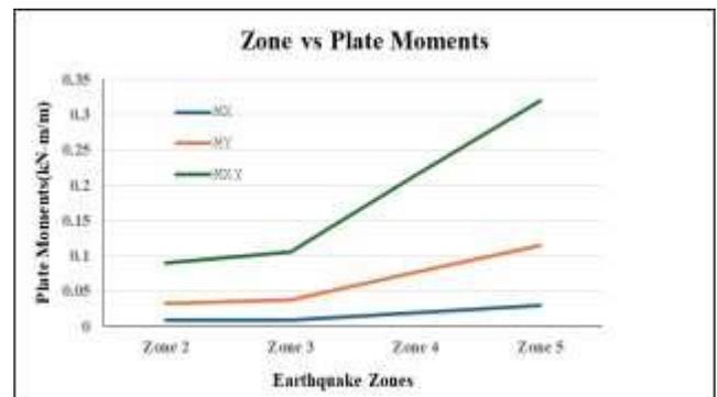
**Fig. 10.4: Plate Moments across varying Earthquake Zones**
