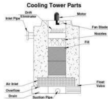
Fig: Components of Cooling Tower
