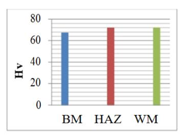
Micro Hardness Test (Sample B)
