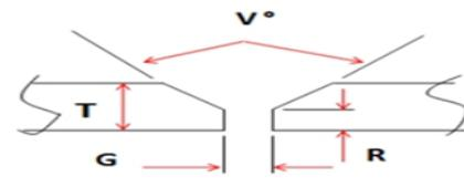
Single V butt welding joint with particulars
