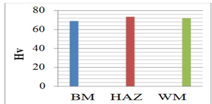
Micro Hardness Test (Sample C)
