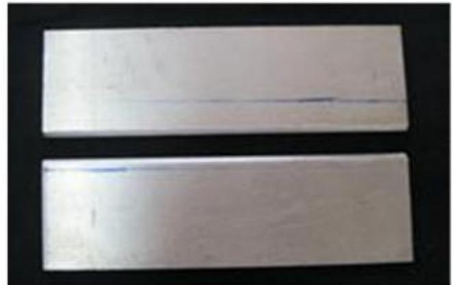
Work piece with Single V butt joint
