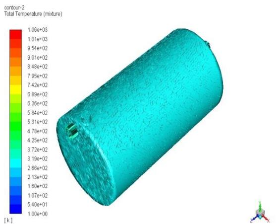
**Figure- 16 Total temperature in shell and helical coil for cold fluid**
