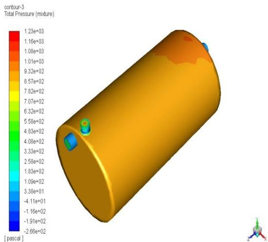
**Figure-8 Total Pressure in shell and helical coil for cold fluid**
