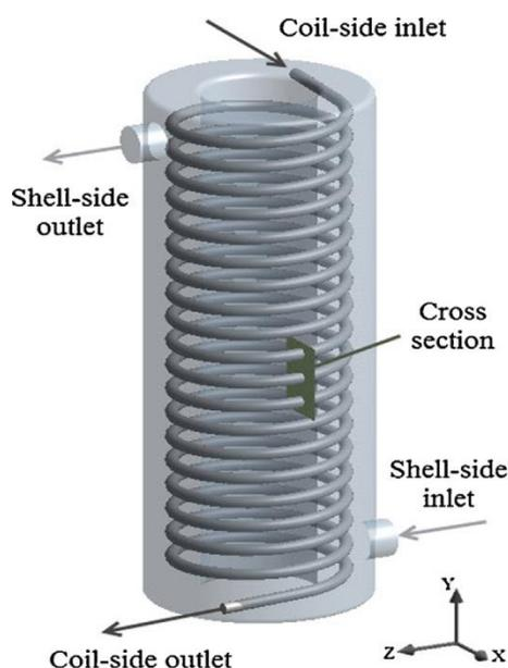
**Figure 1 : Shell and Helical Coil Heat Exchanger**
