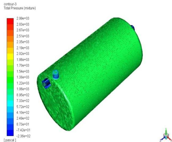
Figure-6 Total pressure in shell and helical coil for cold fluid
