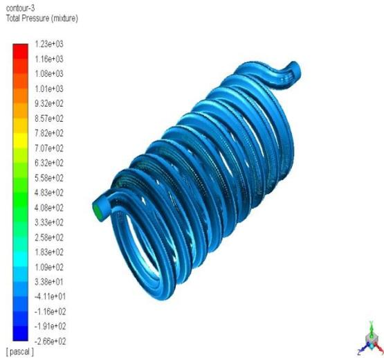
**Figure-7 Total Pressure in shell and helical coil for hot fluid**
