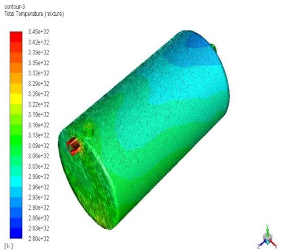
**Figure-12 Total temperature in shell and helical coil for cold fluid**
