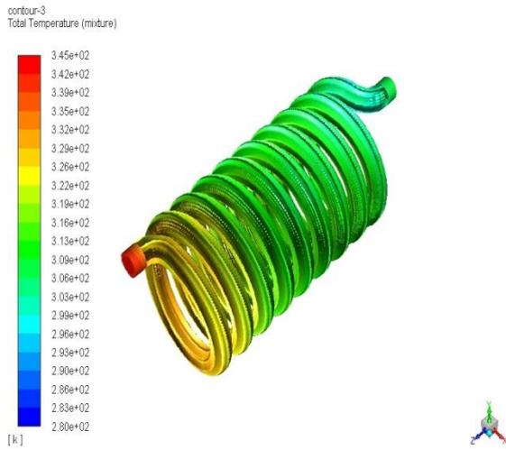
**Figure-11 Total Temperature in shell and helical coil for hot fluid**
