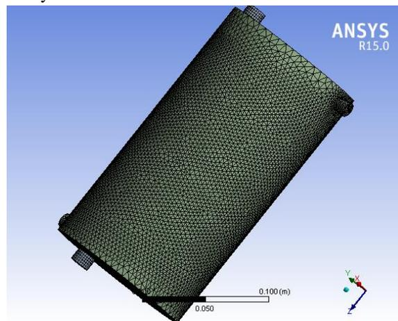
**Figure 4.2: Meshed model with of shell & helical heat exchanger.**
