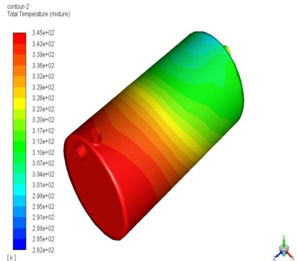
**Figure- 14 Total temperature in shell and helical coil for cold fluid**
