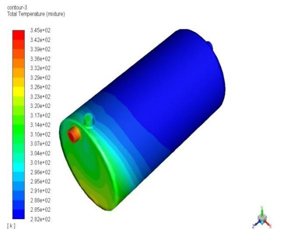
**Figure- 18 Total temperature in shell and helical coil for cold fluid**
