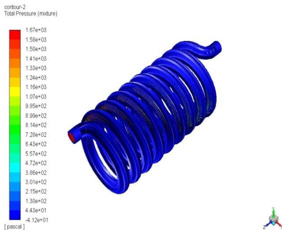
Figure-3 Total pressure in shell and helical coil for hot fluid
