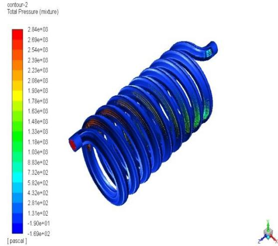
**Figure-9 Total Pressure in shell and helical coil for hot fluid**
