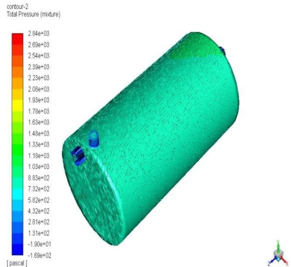
**Figure-10 Total Pressure in shell and helical coil for cold fluid**
