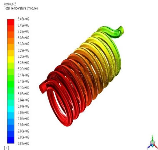
**Figure- 13 Total temperature in shell and helical coil for hot fluid**
