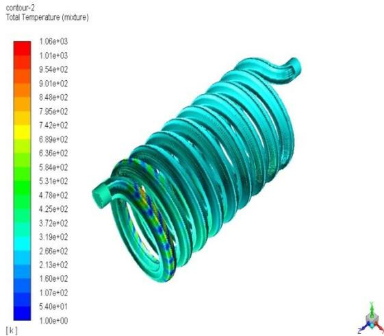
**Figure- 15 Total temperature in shell and helical coil for hot fluid**
