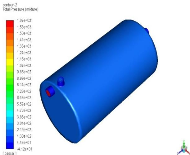
Figure-4 Total pressure in shell and helical coil for cold fluid
