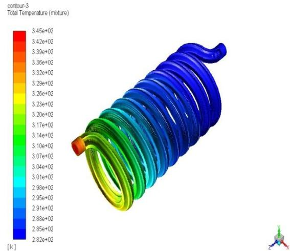
**Figure- 17 Total temperature in shell and helical coil for hot fluid**
