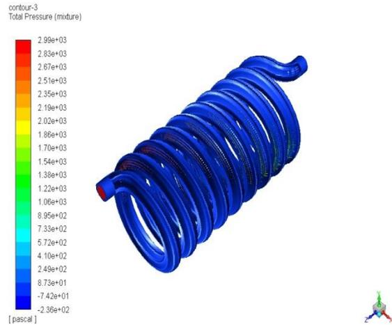
Figure-5 Total pressure in shell and helical coil for hot fluid
