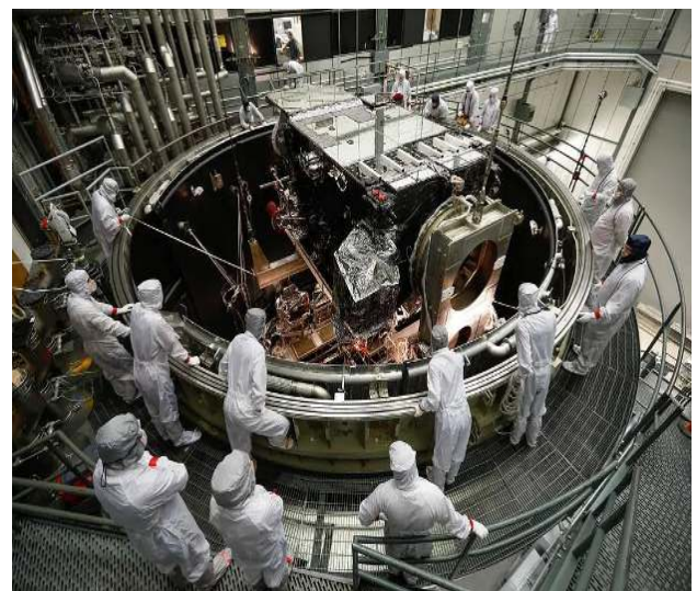
Fig.9. In March, GOES-S was lifted into a thermal vacuum chamber to test its ability to function in the cold void of space in its orbit 22,300 miles above the Earth. (Credit: Lockheed Martin)
