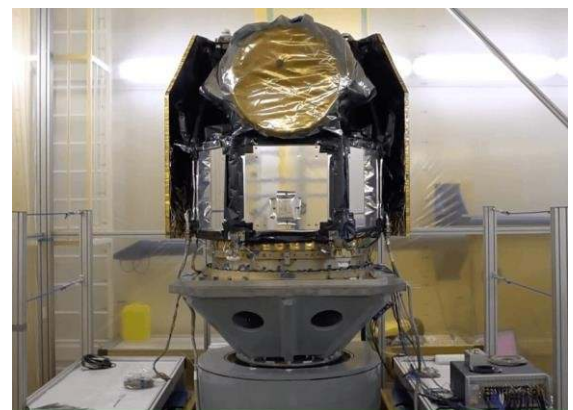
Fig.1. Launch vibration test of ESA's CHEOPS planet-hunting space telescope (Credits:ESA)
