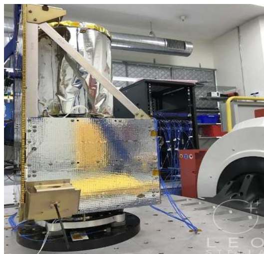
Fig.5. LeoStella's microsatellite is tested on a shaker with m+p Vibcontrol software and m+p VibRunner hardware. To ensure maximum safety, excessive vibration amplitudes are identified and avoided by vector notching. | Photo source: LeoStella
