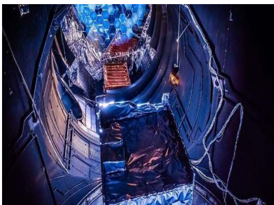
Fig.2. JUICE, ESA's Jupiter-bound spacecraft, is undergoing a high temperature test in a thermovac chamber. Credits: ESA/M. Cowan.
