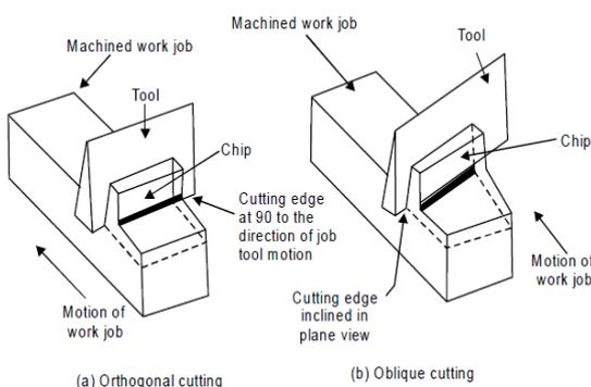
Fig -3: Types of metal cutting
