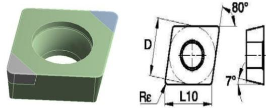
Fig -5: Carbide tool insert
