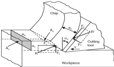
Fig -2: Mechanics of machining
