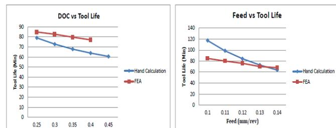
The results showed that the tool life is decreasing as the cutting force, MRR and cutting speed increases. Also tool life is decreasing with increase in speed and feed. Same behavior has been observed with theoretical calculation as well as by FEA.
