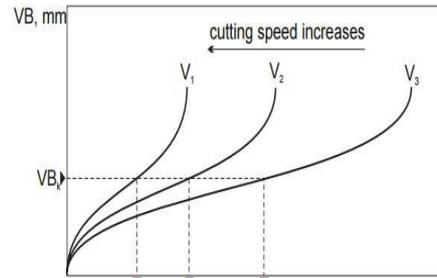
**Fig -1:** Relationship between flank wear criteria and the tool life for diff. cutting speed
