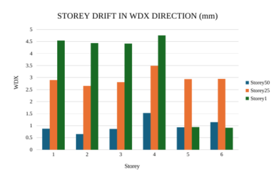
Figure 8. Original report Graph 4.3: storey drift in the WDX direction
