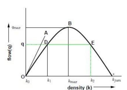
This graph indicates the macroscopic fundamental (is type of traffic flow that relates space-mean flow, density and speed) diagram of traffic flow is a diagram that gives a relation between road traffic and the traffic density.
