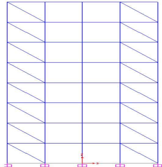
3. Figure 3-D and Elevation View of Eccentric Braced Frame Structure
