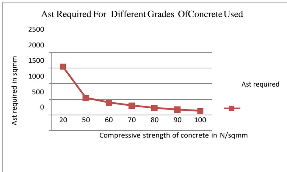
**Graph 3.1. Variation of steel area required with increase in the strength of concrete to be used**
