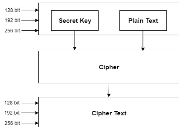
The AES encryption algorithm defines numerous transformations that are to be performed on data stored in an array. The first step of the cipher is to put the data into an array, after which the cipher transformations are repeated over multiple encryption rounds.
