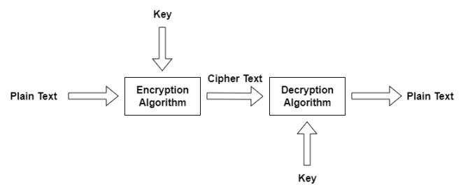
The plain text denotes the text that has been send to the other users on the chat app. The plain text is easy to see and can be read by anyone. The plain text is then converted to Cipher Text using AES Cryptographic Algorithm. And all the cipher text then will be stored on the Firebase database. As all the Text is already converted to cipher text so no one will be able to read it as it will be in gibberish.
