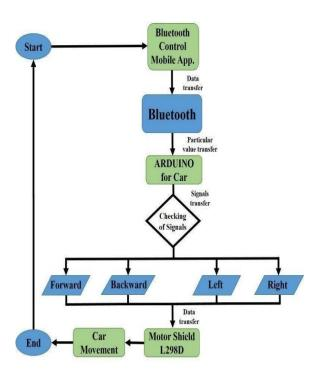
Flow diagram to control robot car with mobileapplication
