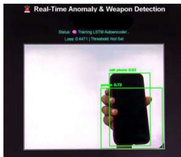
Fig 7.2 LSTM Autoencoder training in progress. YOLO detects persons and cellphone.
