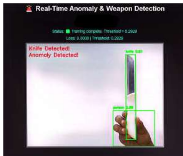
Fig 7.3 LSTM detects anomaly — knife identified.
