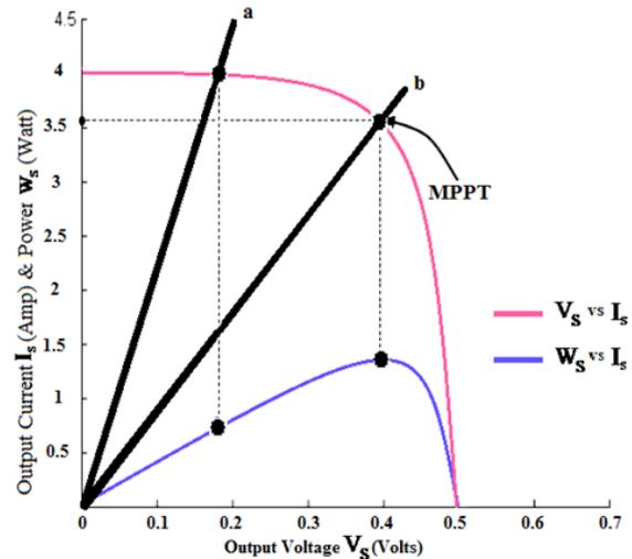
Fig. 4.1 Operating Point of PV Array
