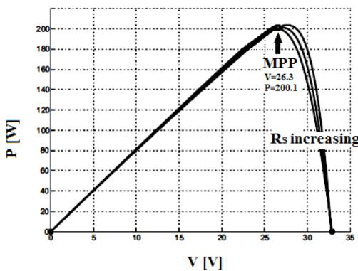
Fig. 3.6 P-V curves plotted for different values of  $R_s$  and  $R_p$
