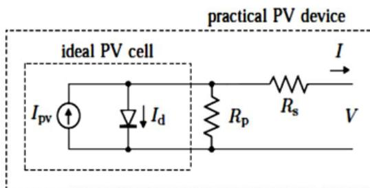
Fig.3.4 Single Diode Model
