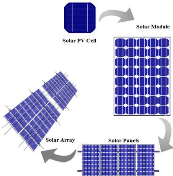
Fig.3.2 PV Cell, Module Array
