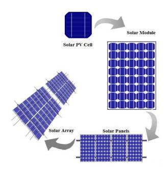
Fig.3.2 PV Cell, Module Array
