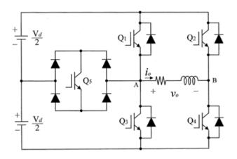
Fig.4.7 Configuration of the proposed single-phase fivelevel PWM inverter
