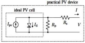
Fig.3.4 Single Diode Model
