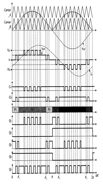
Fig 4.1 Switching patterns of the proposed single-phase five-level PWM inverter
