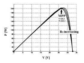
Fig. 3.6 P-V curves plotted for different values of  $R_{\rm S}$  and  $R_{\rm P}$
