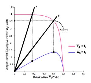
Fig. 4.1 Operating Point of PV Array
