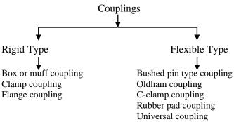
Rigid couplings are employed where shafts are properly aligned. Flexible couplings take care of small misalignment in the shaft axes, either lateral or angular, depending on the type of coupling.
