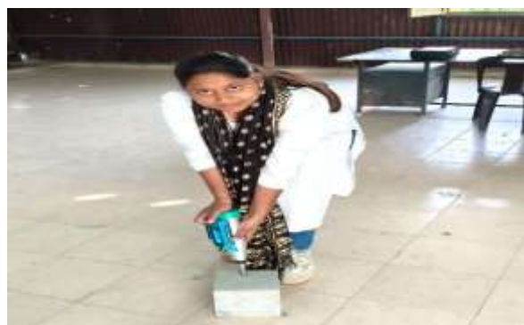
Fig 8: Rebound Hammer Test
