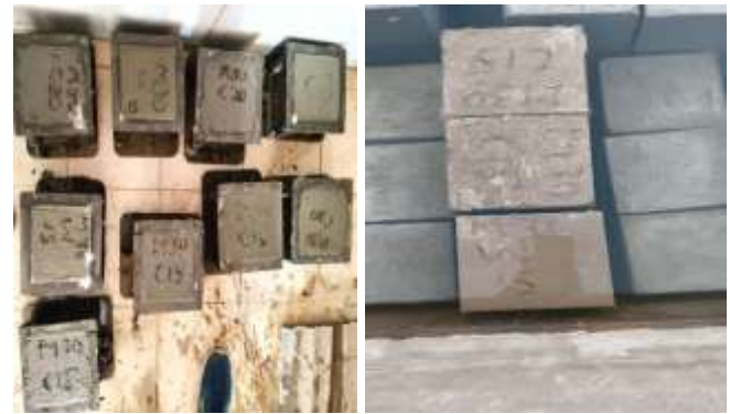
Fig 9: Cube Casting & Curing
