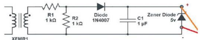
Figure 7. Voltage measurement circuit
