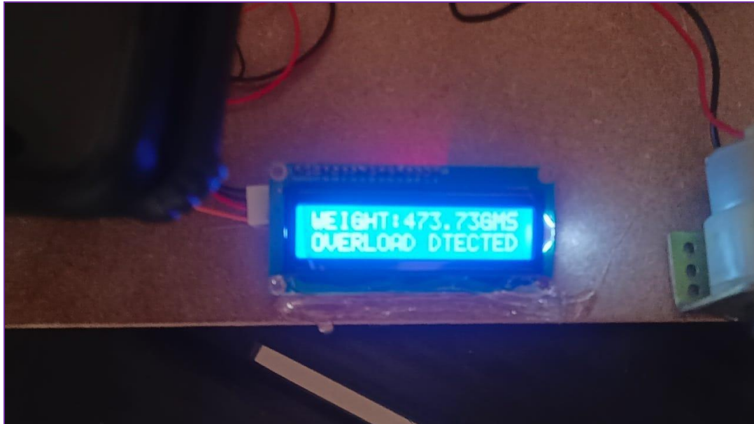
Fig 11 Load cell Weight is greater than Threshold value
