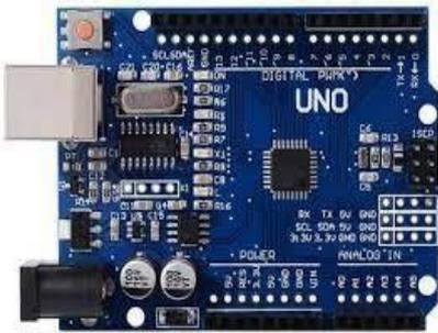
Arduino UNO is also a low- value, flexible, and easy-to- use programmable open- supply microcontroller board which will be integrated into a spread of electronic comes. This board are associated with different Arduino boards, Arduino shields, and raspberry-Pi boards and may management relays, LEDs, servos, associated motors as an output.
