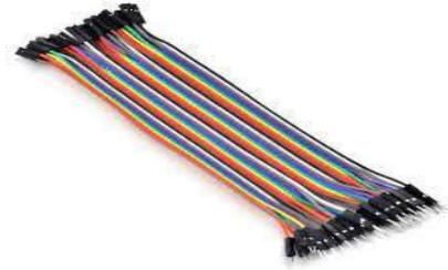
Jumper cables area unit merely cables that have connection pins at every finish, permitting them to be used to connect 2 points to each alternative while not attachment. Jumper wires area unit typically used with breadboards and alternative prototyping tools thus on produce it straightforward to change a circuit as demanded.
